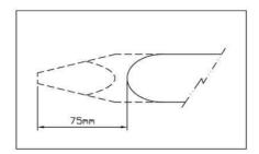
In case Tool is pushed in by continuous hitting on hard rocks
