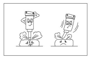
Do not try to break too much at one time. It is wiser to start from the edge and work towards the center.
