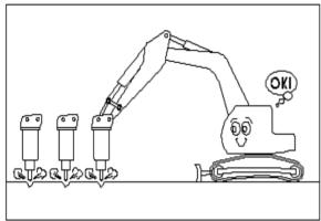
When breaking large rocks, do not attempt to break them from the center. It is more efficient if breaking is done from the edge. Takes small bits and do not work on one spot for more than 30 seconds. This method will increase your productivity and cause less wear and tear on your equipment.
