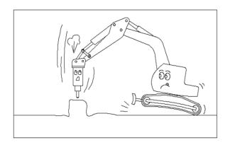
Applied pressure should not lift the carrier high off the ground. As the hammer breaks through the material, the excavator will drop suddenly and harmful shock loads will be transmitted to the tool, power cell and excavator. If the hammer is too heavy for the carrier, the resulting damage will be worse. So it is important to proper size of the hammer to the carrier.
