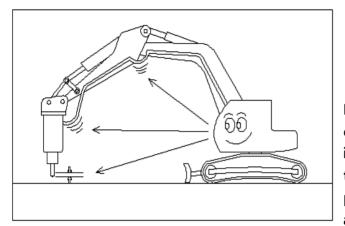
Abnormal surging means the nitrogen accumulator is empty. Stop the hammer immediately and repair the accumulator.
