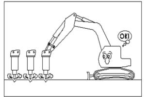
When breaking large rocks, do not attempt to break them from the center. It is more efficient if breaking is done from the edge. Take small bits and do not work on one spot for more than 30 seconds. This method will increase your productivity and cause less wear and tear on your equipment.
