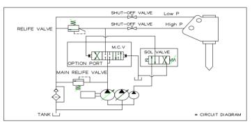
8) After installation of hydraulic pipe lines, check the pressure and oil capacity. Check the relief valve on the hydraulic system, which secures high pressurized accumulator. It must have been approved by the relevant authority. Make sure that the pressure of relief valve has been set correctly, i.e. to the maximum permissible operating pressure of the hydraulic hammer.
