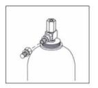
(3) Open the main valve of gas charging cylinder counterclockwise to reach the pressure gauge to optimum pressure. Close the cap clockwise to stop the gas filling.
