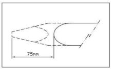
In case Tool is pushed in by continuous hitting on hard rocks Damage to upper part of Tool by excessive abrasion of Tool Holder Bushing
